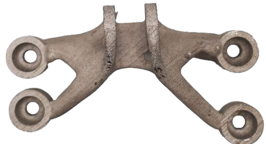
Exemplary Additively Printed Aviation Component [courtesy of Plastometrex]
