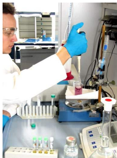
Determination of water hardness by titration
