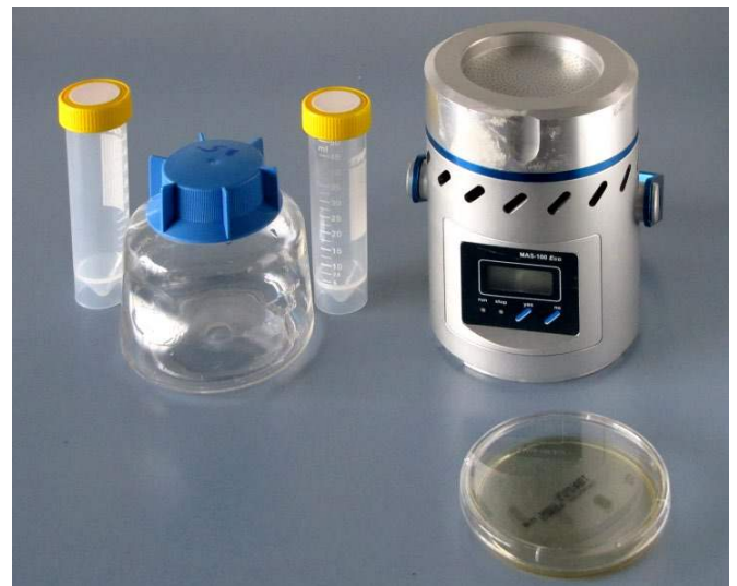
Equipment for taking samples for water analysis and bacterial indoor air measurements
