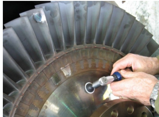
Ambulant metallography on a stationary gas turbine
