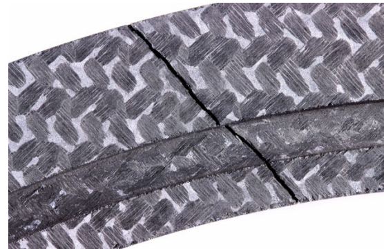
Fracture in a carbon fibre reinforced component
