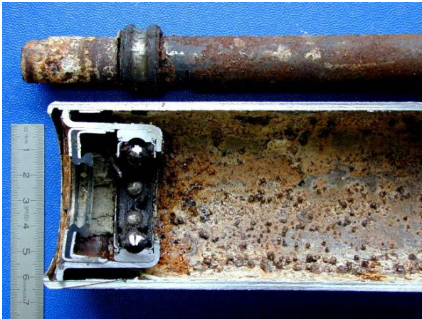
Corrosion damage to the roller of a conveyor belt
