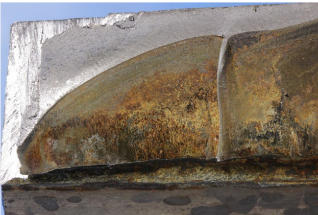
Vibration fracture in the cylinder block of a gas compressor, caused by a corrosion attack in the cooling water channel (macrophotography)
